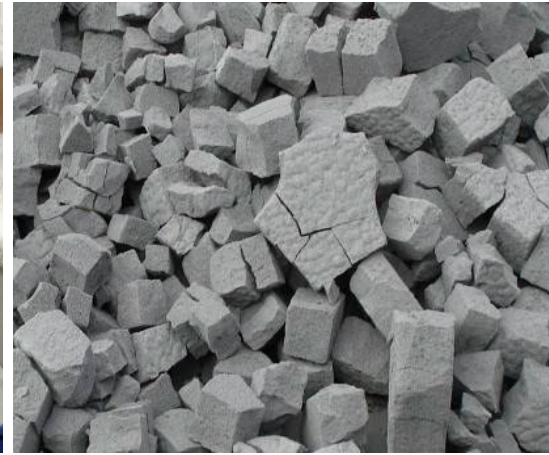
Example Foam Glass Gravel Load bearing insulation under ground slabs
