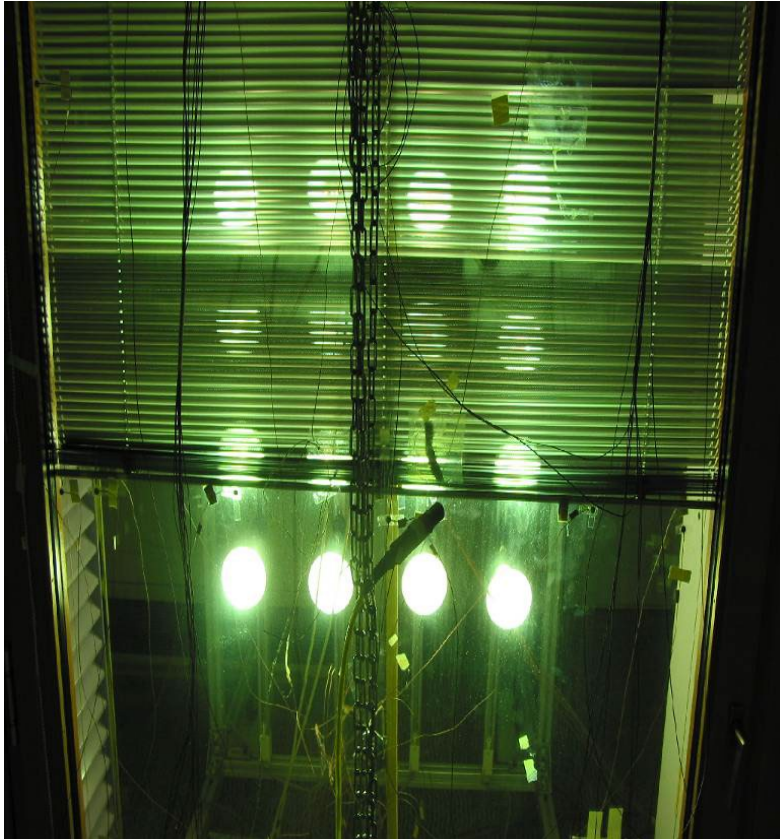
Blinds in the gap of double glazing are tested with high temperature differences
