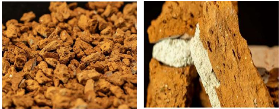
Figure 1 Photos of masonry rubble by [ 45 ] fragments with firmly adhering mortar residues, right, masonry rubble is mostly made up of brick, left: via an automated sorting process, brick and mortar rubble can be separated from each other.
