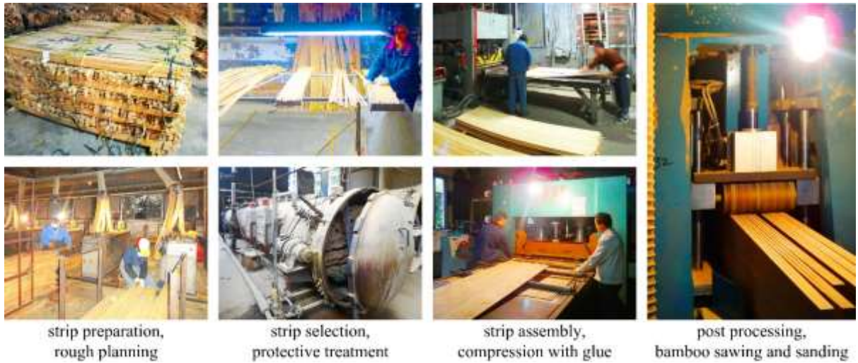
Figure 1: Photos of laminated bamboo production.
