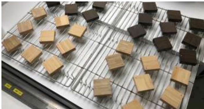
specimens (size: 5×5×1.35 cm), with four sides and bottom surface sealed
