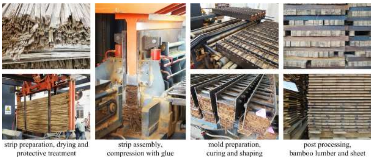
Figure 3: Photos of bamboo scrimber production.
