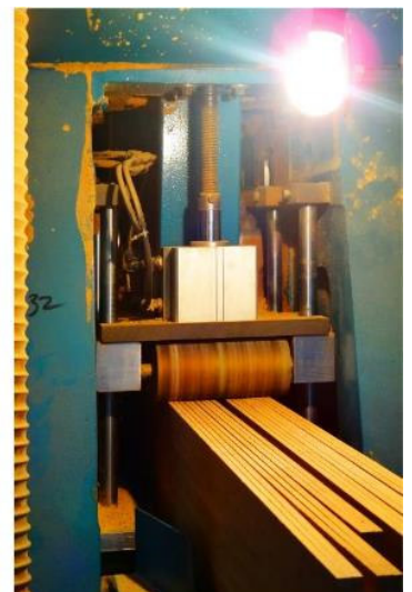
post processing, bamboo sawing and sanding
