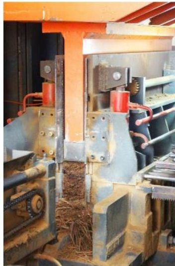
strip assembly, compression with glue
