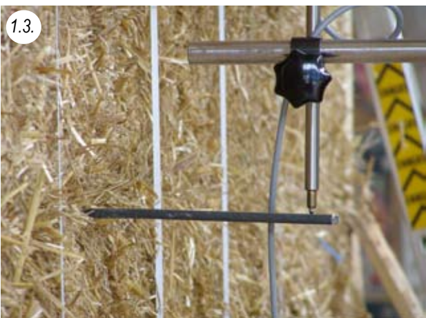
Sensor for force-deformation diagram
