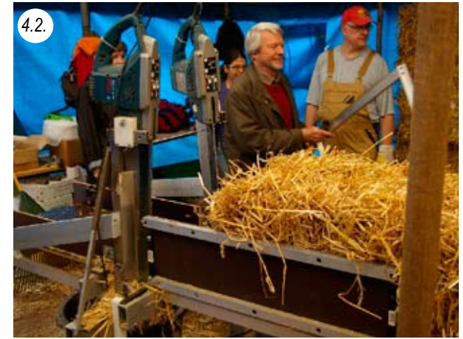
Device to cut the bales conically, (high precision is necessary)
