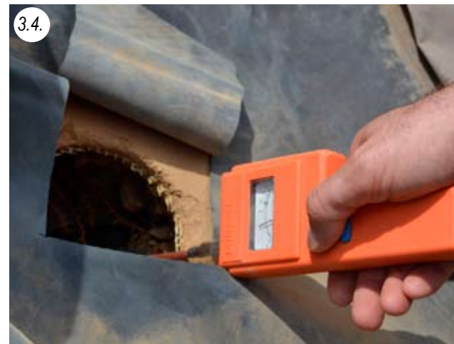
Structure: Clay plaster on the inside on straw bales, clay on the outside, then pond liner and grass roof. No condensation (!) - hard to believe in terms of building physics...
