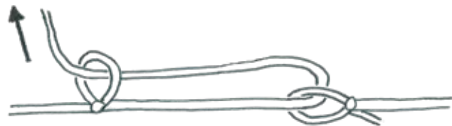
Block knot, high tension possible
