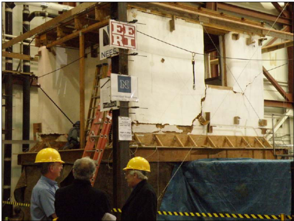
Figure 7. Damage to the house after 0.82g (200% Canoga Park)
