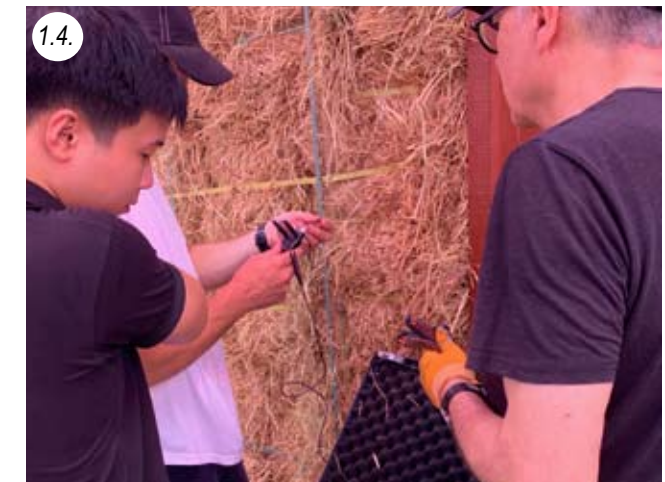
Installation and calibration of moisture sensors
