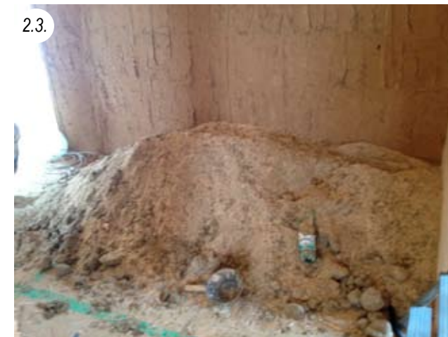
2.3. Light clay - loamy excavation + sawdust (e.g. 1:1 volume)
