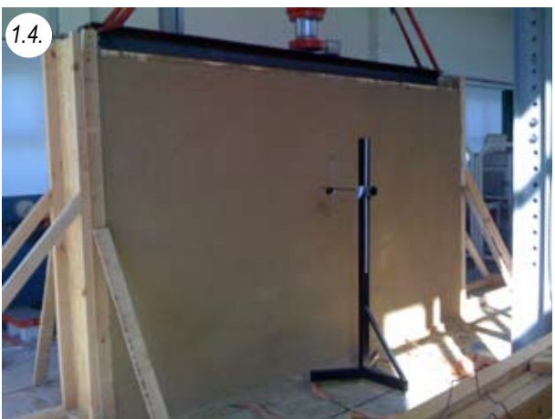
Test wall in plastered condition
