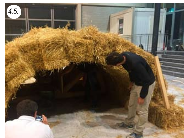
Static experiments with students from the Salzburg University of Applied Sciences no conically cut bales were used
