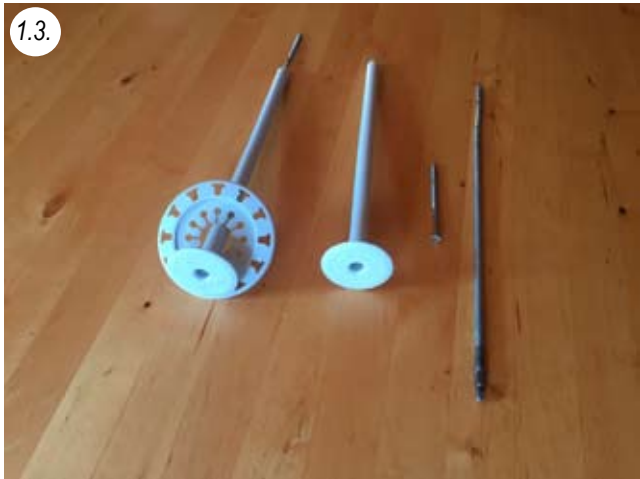
Insulation anchor FA WKRET-MET, 285 mm long, in combination with special 90 mm screw perfect for bale thickness, + extended Torx bit. For mounting the bales on the outside wall.
