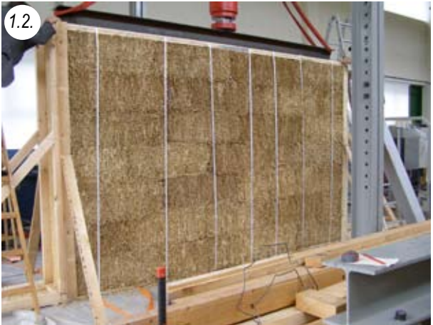
Test wall unplastered
