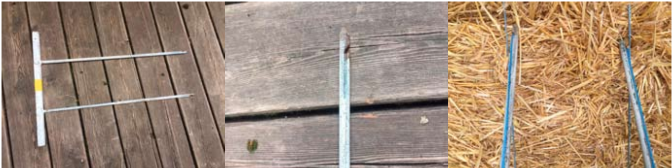
Baling needle in double design Needle point with notch for piercing the cord through the bales Completely threaded cords - for both new bales, therefore double the cord
