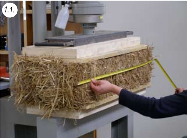
Single bale tests up to 35 KN
