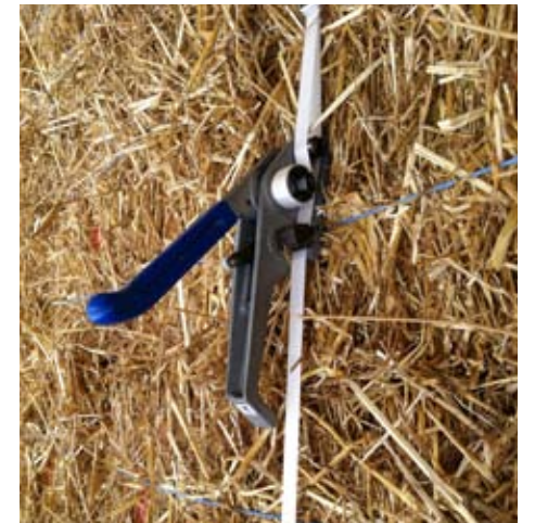
Clamping device in use, also useful for facades to close joints and prevent settlement
